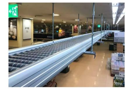
The system integrator LG CNS in Korea, a customer of Avancon, installed the conveyors under the roof. Avancon conveyors are light weight because they are made all of aluminum anodized, perfect for hanging under the ceiling, they look clean and streamlined, perfect for shown in public.
