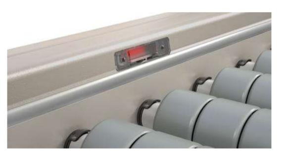
All light barriers of a subsystem communicate with a master and signal whether a zone is occupied or empty. This enables conveying without the conveyed goods touching each other.
